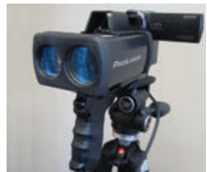
The speed monitoring equipment.
