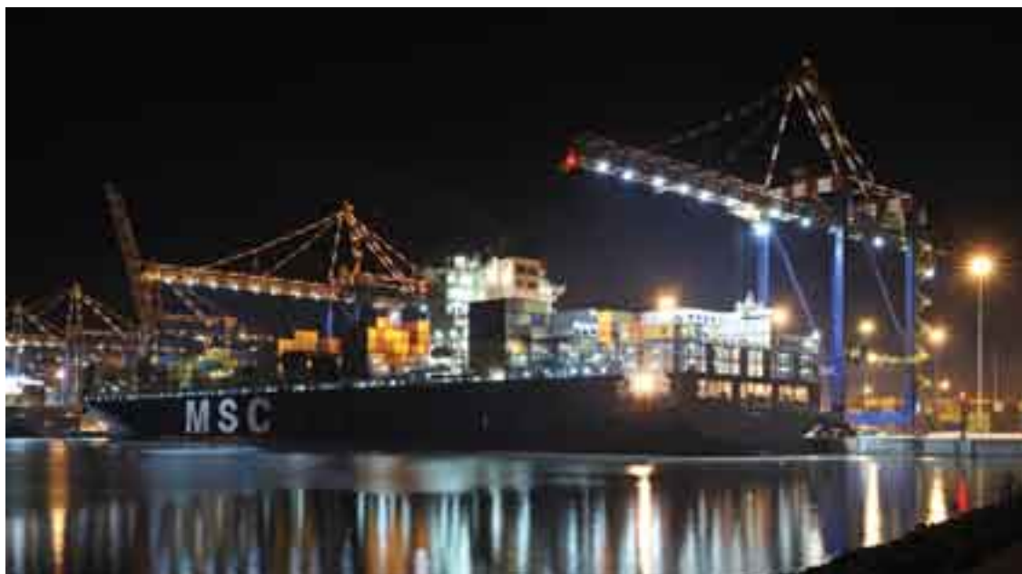
Big movers – the biggest vessel to call on South Africa to date, the 336-metre-long, 9 000-TEU MSC Chicago berthed in Ngqura, which was its first port of call in Africa.
