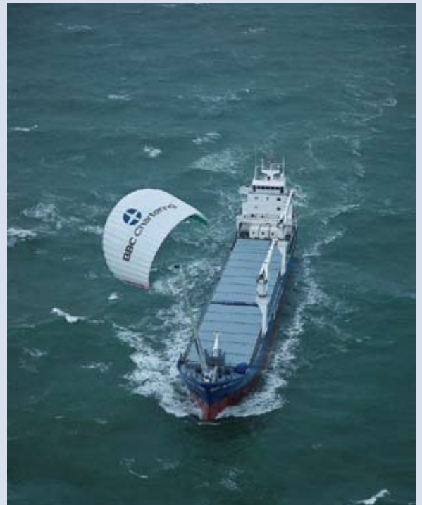
Wind propulsion system uses a kite to deliver engine load relief.
