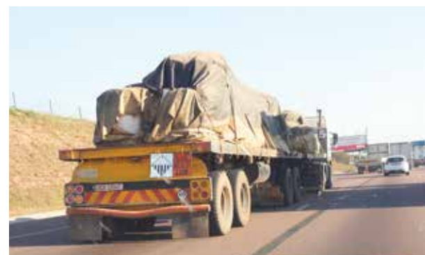
This truck, photographed on the N1, is in blatant contravention of several dangerous goods transport regulations, including the fact that the placarding identifying the hazard of the cargo is both upside down and defaced.
