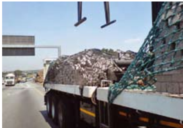
A poorly secured load of bricks
